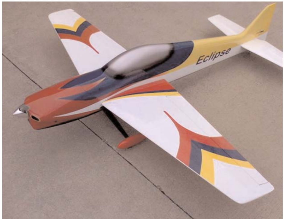
This is Forest Wilhite's first pattern ship that he built. I here it weighs in around 10 and 1/2 pounds and he flies it with a YS160. Yup it has unlimited vertical.
