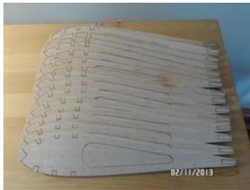
Once all the ribs are notched and lightened, lay them up into a stack to check the alignment of the notches for the stringers, LE, TE and lightly sand where needed to align without oversizing the notches. I use a 1/8" aluminum bar wrapped with sanding bar paper to achieve this.
