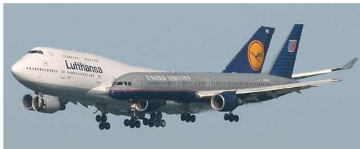
A Lufthansa 747-400 and a United 757-200 are on a simultaneous landing approach on the parallel runways 28L and 28R at San Francisco International Airport. Real runway separation is only 225 meters.
